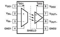
A 0.1 µF bypass capacitor must be connected between pins 1 and 4 and between pins 5 and 8.
